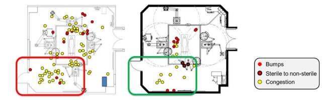
*Figure 4*. Comparison of bumps and congestions between the initial mock-up design iteration (left) and final mock-up design iteration (right) when enacting the laparoscopic cholecystectomy scenario.
