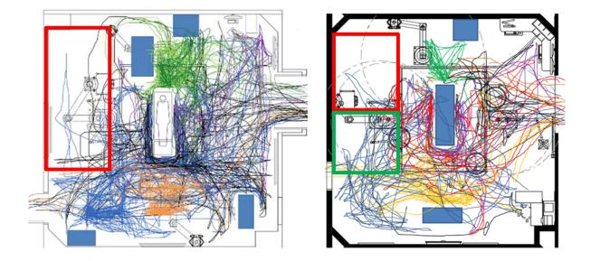
*Figure 7*. Link analysis of the laparoscopic cholecystectomy scenario enactment indicated that the amount of under-utilized space in the room (red box) decreased in the final mock-up design iteration (right) compared to the initial mock-up design iteration (left).
