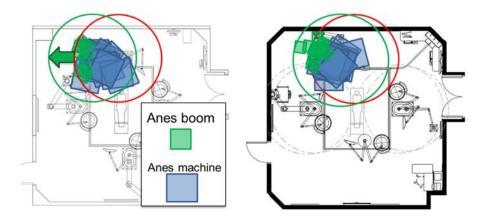
*Figure 5*. Placement of the anesthesia boom and anesthesia machine was examined by plotting their various locations across scenarios in the initial mock-up design iteration (left) and final mock-up design iteration (right).
