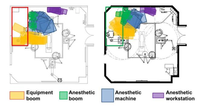
*Figure 8*. Visual representation of equipment and booms placement across scenarios where video analyses were conducted in the initial mock-up design iteration (left) and final mock-up design iteration (right).
