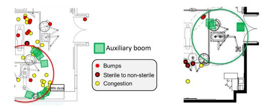
*Figure 6.* Comparison of congestions in the initial mock-up design iteration (left) to the final mock-up design iteration (right) suggested that access to the nursing station was improved; there was less congestion in the space around the nursing station. Furthermore, the potential range of motion of the auxiliary boom in the final mock-up design iteration (green circle), included the full length of the OR table, which was not the case in the initial design (red circle).
