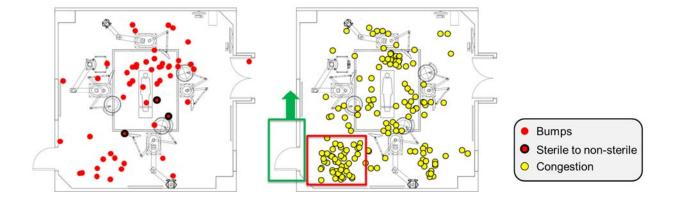
*Figure 3.* Bump analysis (left) and congestion analysis (right) are based on observations coded during the video analysis across the three scenarios. Congestion near the entrance (red box) informed the recommendations to relocate the door and pass-through (green box and arrow).
